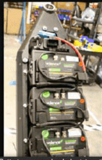
Batteries are loaded into the extruded aluminum chassis of the Brammo Eneria. The frame also acts as the battery tray. With three batteries mounted above and three mounted below.
